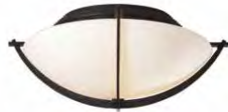
COMPASS FLUSH MOUNT - 124550 US PATENT D 592,796 - 6.4" h x 15.7" dia - 8" OD canopy 6.4 lbs - Medium sockets (2), 60 W max, A19 bulbs
