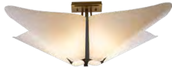
KIRIGAMI SEMI-FLUSH - 123305 - US PATENT D660,501S 8.5" h x 22.5" sq - 4.5" sq canopy - 5.7 lbs Medium sockets (4), 60 W max, A19 bulbs
