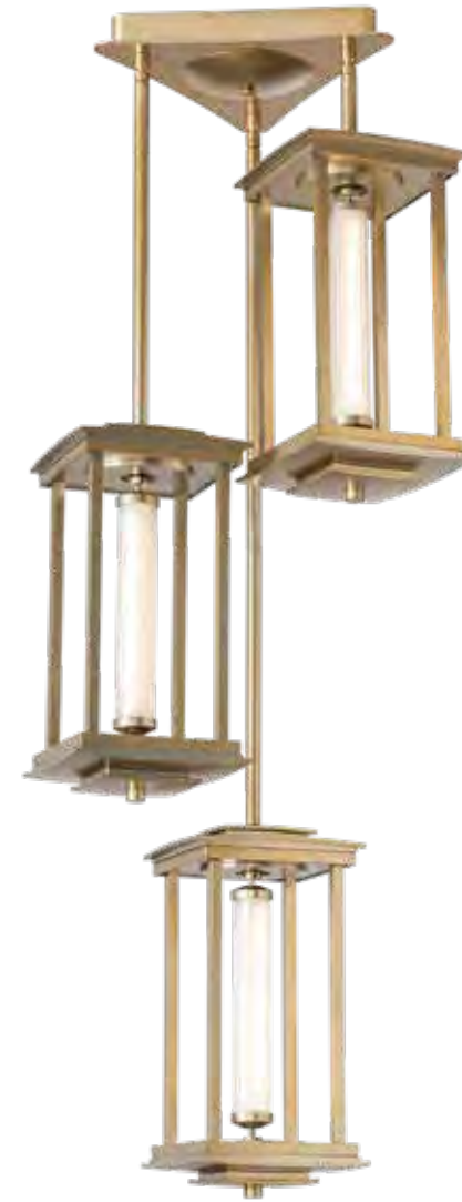
NEW ATHENA TRIPLE SHORT LED LANTERN - 131635 15.2" h x 20.1" dia - 9.7" tri canopy - 120" wire - 11 lbs 1440 EST. DELIVERED LUMENS, (3) 4.3W, 3000K CCT, 90 CRI, 120V INPUT, DIMMING: ELV, TRIAC, 0-10
