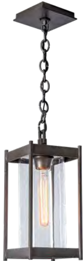
NEW CELA MEDIUM OUTDOOR LANTERN - 362021 14.1" h x 6.2" sq - 27.9" OAH - 5.3" sq canopy - 1' chain 5' wire - 4.6 lbs - Medium socket, 100 W max, A19 bulb
