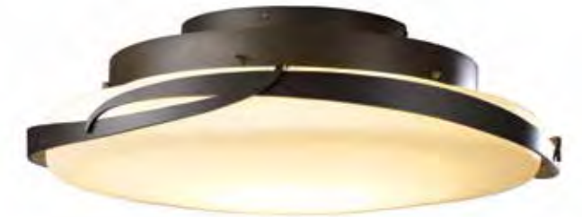
FLORA LARGE LED FLUSH MOUNT - 126742 7" h x 24.1" dia - 10" OD canopy - 25.9 lbs 1400 EST. DELIVERED LUMENS, 1-28W, 3000K CCT, 93 CRI, 120V INPUT, DIMMING: LINE VOLTAGE, ELV, TRIAC
