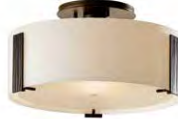
IMPRESSIONS SEMI-FLUSH - 126753 6.1" h x 11.8" dia - 5.25" OD canopy - 4.4 lbs G9 socket, 60 W max, G9 bulb, incl
