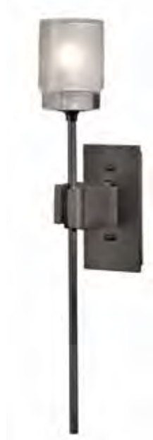
ECHO SCONCE - 204320 16.2" h x 3" w x 3.9" d - 2.8 lbs 3" x 5" backplate - 8.7" vertical mounting ht G9 socket, 60 W max, G9 bulb, incl
