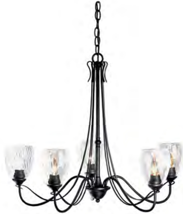
TRELLIS 5-ARM CHANDELIER - 103063 - US PATENT D532,546S 21.9" h x 28.1" dia - 5" OD canopy - 15' wire, 3' chain 7 lbs - Candelabra sockets (5), 60 W max, B bulbs
