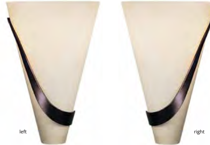
HALF-CONE SCONCE - 206563 12" h x 8" w x 4.2" d - 4 lbs 5.6" X 1" X 9.3" backplate - 7.9" vertical mounting ht Candelabra sockets (2), 60 W max, B bulbs
